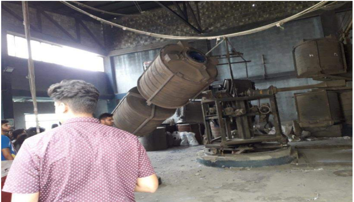
BBA students of Tecnia Institute of Advanced Studies, Delhi able to understand the functioning of Bi-Axial rotomoulding Machine on 16.09.2019
